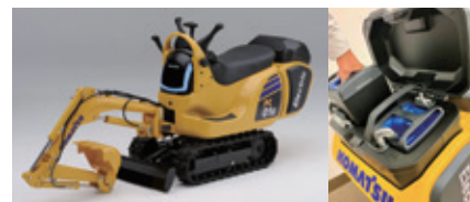
Komatsu Ltd.'s PC01E-1 electric micro excavator fitted with an Honda Mobile Power Pack
