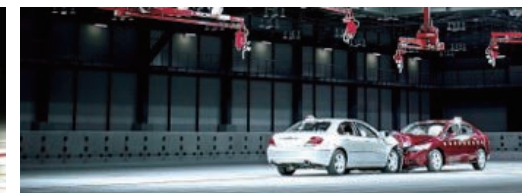
Indoor omni-directional crash test facility
