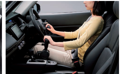
An example of a vehicle equipped with Honda Techmatic System Type D (manual driving assist device)
