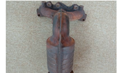
Cracked exhaust manifold of Honda Life mini-vehicle made in 1999
