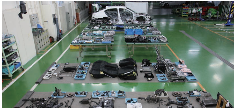
Verification of parts following durability testing
