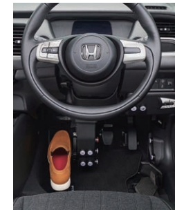
An example of a vehicle equipped with Honda Franz System (steering pedal)
