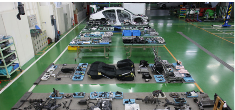
Verification of parts following durability testing
