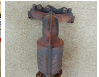
Cracked exhaust manifold of Honda Life mini-vehicle made in 1999
