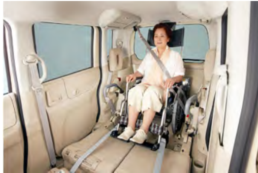
Artist's conception of a passenger in a wheelchair in a wheelchair-accessible N Box+
