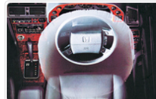
Honda equipped the 1987 Legend with the first airbag system to be used on any domestically produced vehicle
