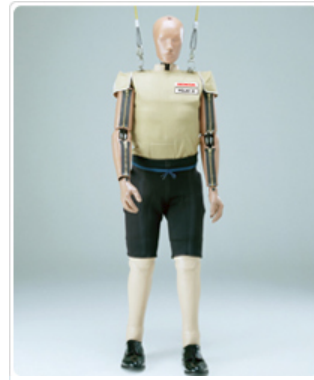
The POLAR III third-generation pedestrian test dummy, which embodies the hopes of its developers
