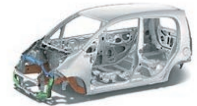
Advanced Compatibility Engineering (ACE) body structure
