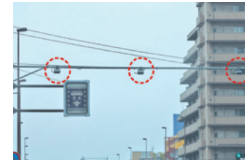
Advanced infrared (IR) beacons installed in Fukuoka City
