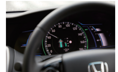
Multi-information display to show guidance to drivers to maintain speed or slow down based on traffic signal data
