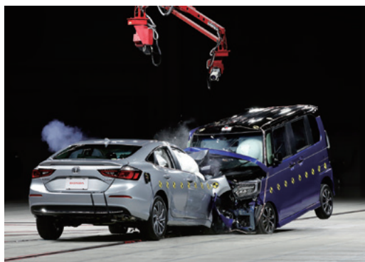
Omni-directional crash test facility
