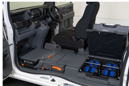
Swappable batteries installed inside the vehicle
